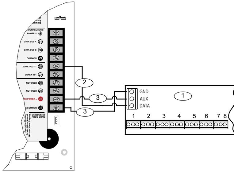
1 - D8129 OctoRelays for relay numbers 1 to 64. Connect OctoRelays in parallel.
