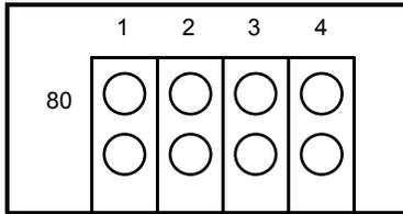
The DX4010i has specific DIP switch settings for SDI Address 80 when home or building automation is desired. *Figure 32* on page 64 shows the correct settings for Address 80.
