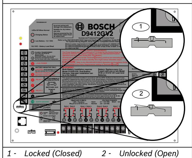
1 - Locked (Closed)    2 - Unlocked (Open)
