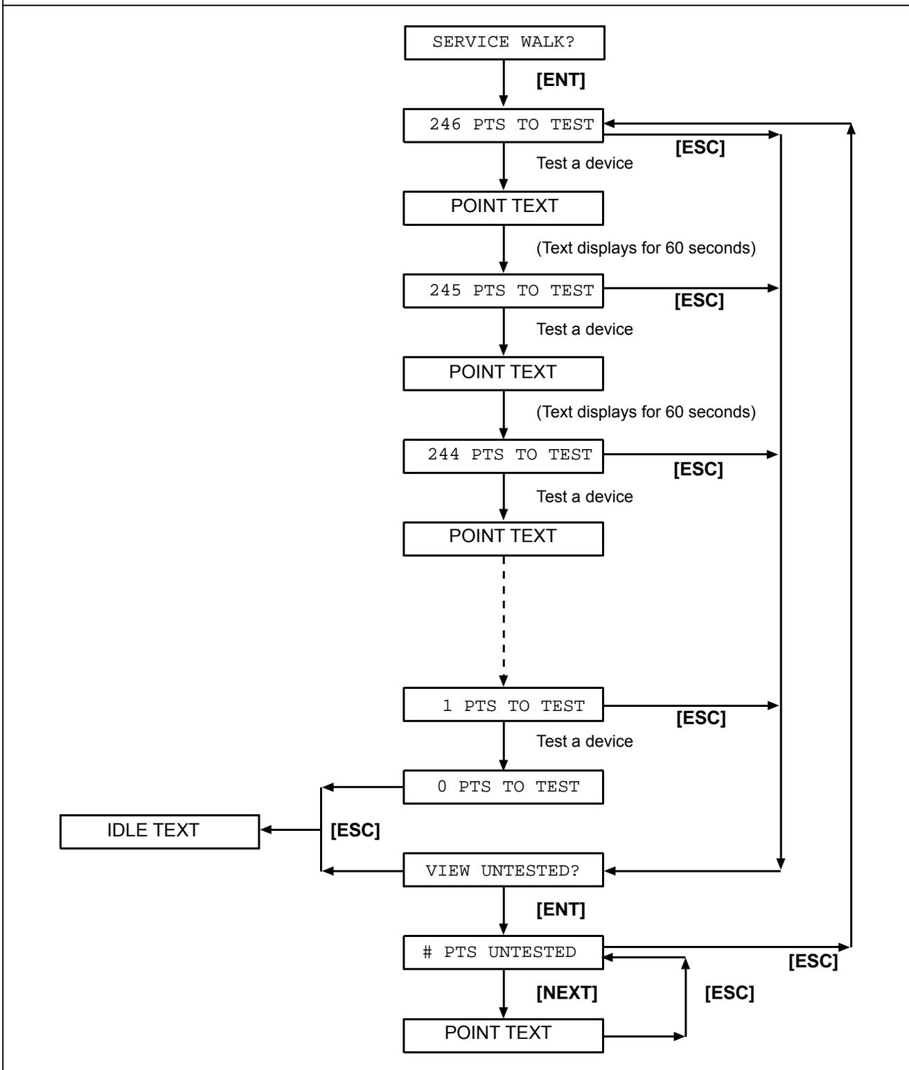
Figure 8: D7412GV2 Service Walk Test Flow Chart
