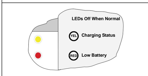
**Investigate Low Battery reports immediately:** If primary (AC) power is off and the discharge continues, the control panel becomes inoperative when the battery voltage drops below 10.2 VDC.
