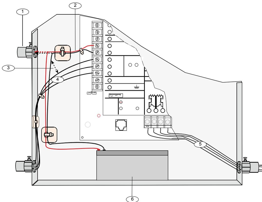
1 - Conduit, required only if external batteries are used.
